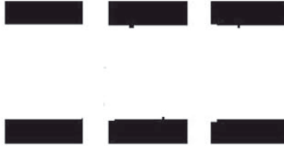
Figure 5. Results from 3 separate runs achieved with two dimensional genetic operators, for bending only so no webs
